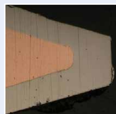
Lötspitzenverschleiß Almit-Lötendraht LFM-23 S Soldering tip wear Almit solder wire LFM-23 S
